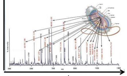
m/z (Mass-to-charge ratio) The ions generated by the irradiation are analyzed by mass spectrometry based on time of flight of the ions.
